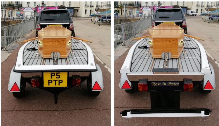
The gunwale at the stern is hinged to enable the coffin to be loaded & unloaded with ease
